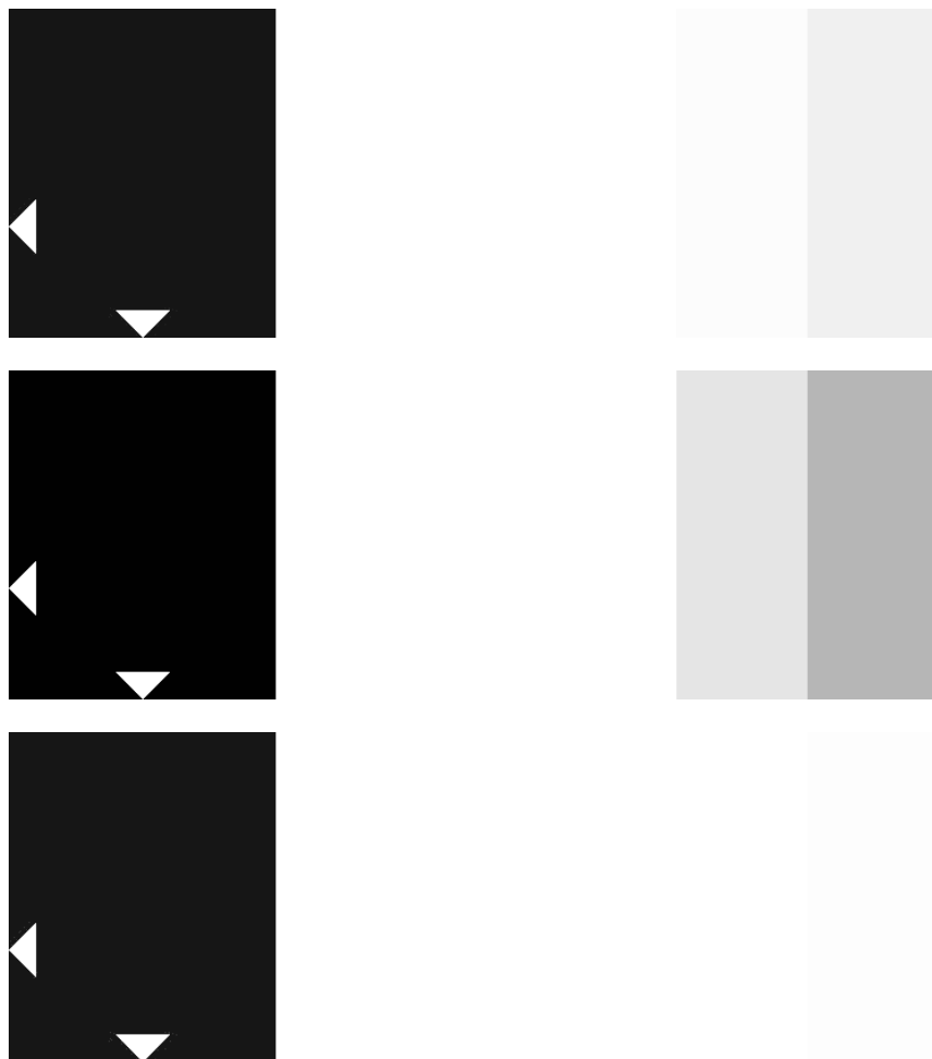
Figure 6.3.2.1 – Above: Here the contrast for extended range is adjusted properly. The bar 2 is minimally brighter than the bar 3. The bar 4 is slightly darker than the Bar 3. Middle: The bars vary significantly. The contrast value is set too low. Below: All the bars have the same brightness. You can't see any differences. The contrast value is set too high.
