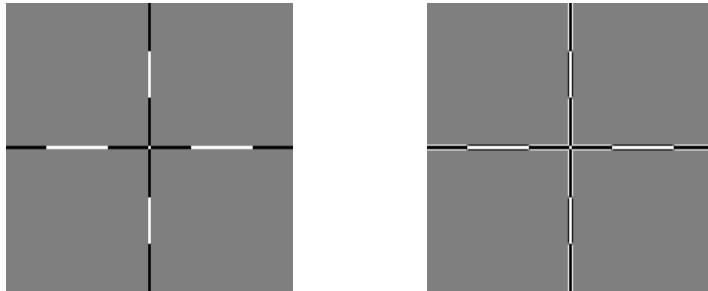
Figure 6.6.1 – Left – correctly set. Right - wrong settings (double contours visible)
