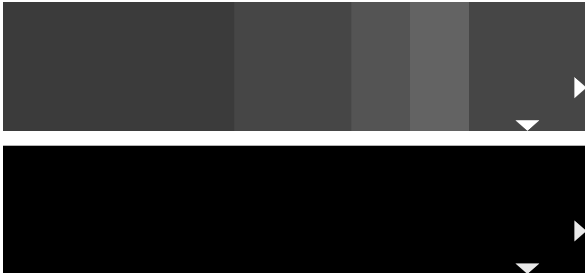
Figure 6.2.2.2 – Above: Here the brightness for extended range is adjusted properly. The bar 3 is minimally darker than the bar 4 and the bars 5 and 6 are slightly brighter than the other bars. Middle: The bars differ significantly, and black appears gray. The brightness is set too high. Below: The bars are not different in brightness. The brightness is set too low.
