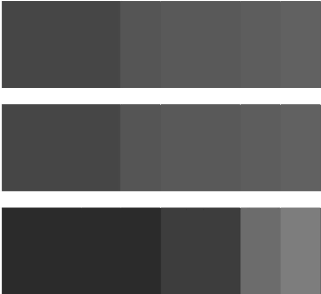
Figure 6.1.2.1 – Top - Full Range. All six bars of the gray scale are visible. Center - Extended Range. Only the bars 3 to 6 are visible. Below - Normal Range. Only the three right bars are visible.
