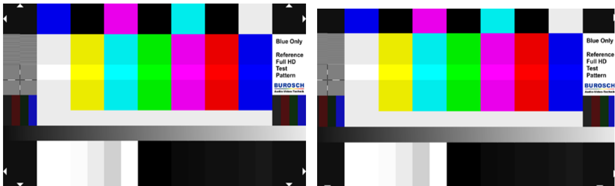
Figure 6.5.2 Gesamtansicht – Left – correctly set. Right - wrong settings (overscan enabled)
