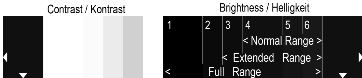
Figure 6.2 – The lower image area of the test pattern to adjust the brightness. The bars 1 to 6 are emphasized for the figure( white lines). Depending on the video range of your display you will see a similar or different representation. Please read the previous chapter. The video range of your display pretends, which bars you have to use to adjust the brightness.
