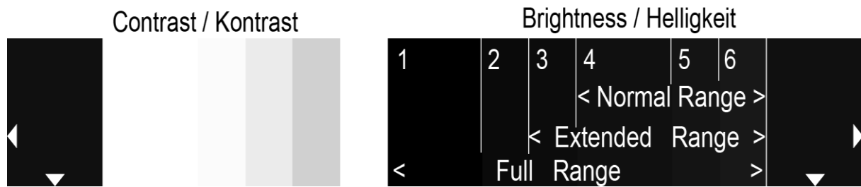
Figure 6.1.2.1 – The black levels - for adjusting the display brightness - can also be used to evaluate the video range of the signal.
