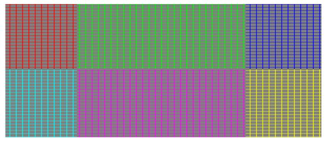
**Vertical lines missing in regular distances and/or remaining vertical lines are broader:** The TV device applies color subsampling in horizontal direction internally without counteracting the negative effects using interpolation. The result is mssing lines and / or broader vertical lines.
