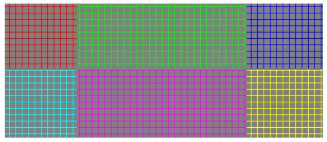
**Big spaces between lines:** In this case, use the white and black sections for comparison. If the spaces in the colored sections are bigger than in the black / white sections, color subsampling is applied internally and no interpolation is applied to counteract the effects.
