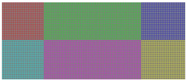
**Horizontal Lines are blurred or darker than the vertical lines:** The TV device applies color subsampling in vertical direction internally and counteracts the negative effects using interpolation.
