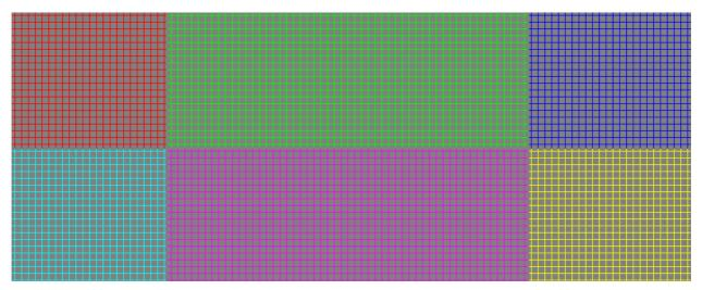
**Optimal Reproduction:** Nothing is wrong with this reproduction. If your display shows the test pattern this way, no internal color subsampling is applied and hence the playback device works perfectly in terms of color subsampling.
