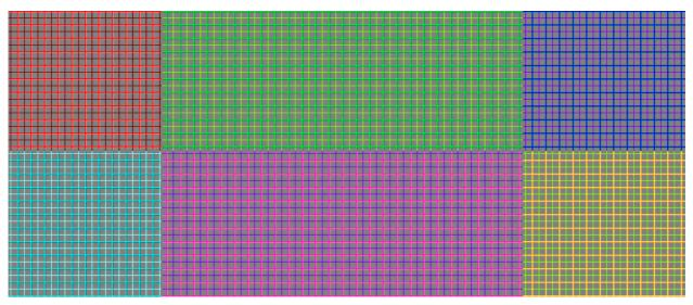
**Similar problems as in the other cases, but limited to one section and/or discoloration:** Your TV display does not apply color subsampling, but shows significant problems in displaying fine colored lines in a pixel exact way. With high probability this is an error in the internal software.
